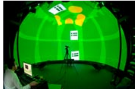
A total of thirteen F22 series projectors are blended into a single image in a military simulation projector. The F22 series, thanks to its small size, and flexible lens configurations, is perfect for this type of application, and reduces complexity and real estate requirements to a minimum. Images courtesy of Air Force Research Lab (AFRL) Mesa, AZ, USA.
