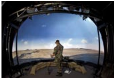
A total of thirteen F22 series projectors are blended into a single image in a military simulation projector. The F22 series, thanks to its small size, and flexible lens configurations, is perfect for this type of application, and reduces complexity and real estate requirements to a minimum. Images courtesy of Air Force Research Lab (AFRL) Mesa, AZ, USA.
